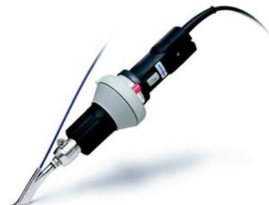
An equally important factor in hot gas (air) welding is the style and type of welding nozzle (tip). Their function is to properly distribute the hot air onto the parent sheet and to heat up and guide the welding rod in the high speed welding process. A variety of tips are available for specific applications. In the field of plastics fabrication, the most common nozzles are the round (freehand), tacking, high speed and the combination high speed welding and tacking tips.
