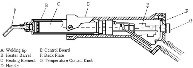
The latest trend in developing electronic controls for hot air heating elements incorporates closed loop controls that hold the temperature constant even while air flow or supply voltages fluctuate.
