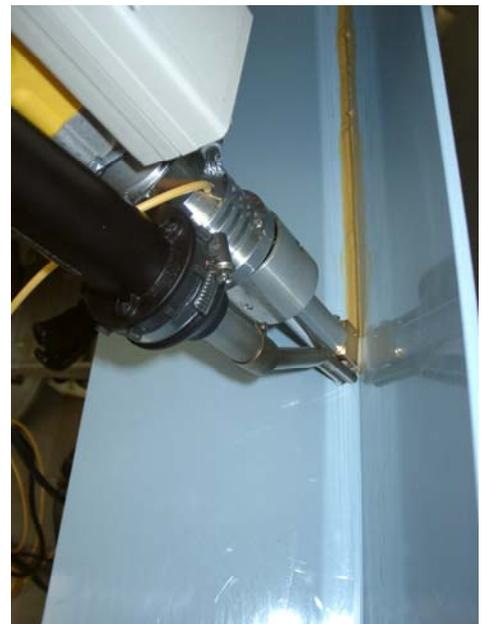
volume air source. When using the self contained machines specific care needs to be taken to assure that the parent material is sufficiently heated.
